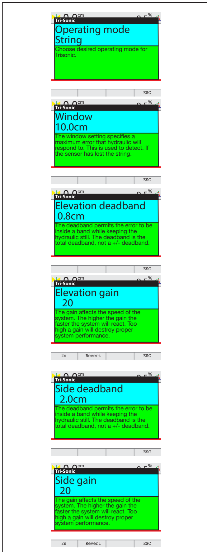
Figure 3-23. Setting up Tri-Sonics.
